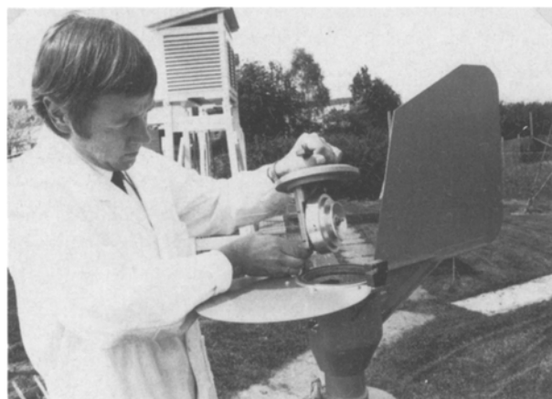
Figure 2. a and b. Pollen trap according to Burkard.
